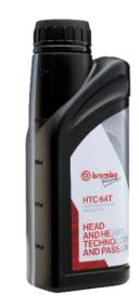
HTC64T has been specifically formulated to provide the highest performance and consistency under all racing conditions, with an extremely high dry boiling point of 335°C (635°F). The higher viscosity of this fluid delivers a stiffer pedal and provides stable performance under extreme temperatures.
