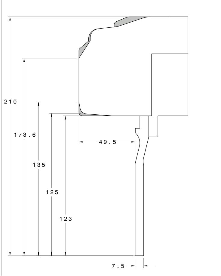
SHADED AREAS INDICATE ADDITIONAL CLEARANCE NEEDED FOR SYSTEMS USING GTR CALIPERS ("R" SUFFIX SYSTEMS)
